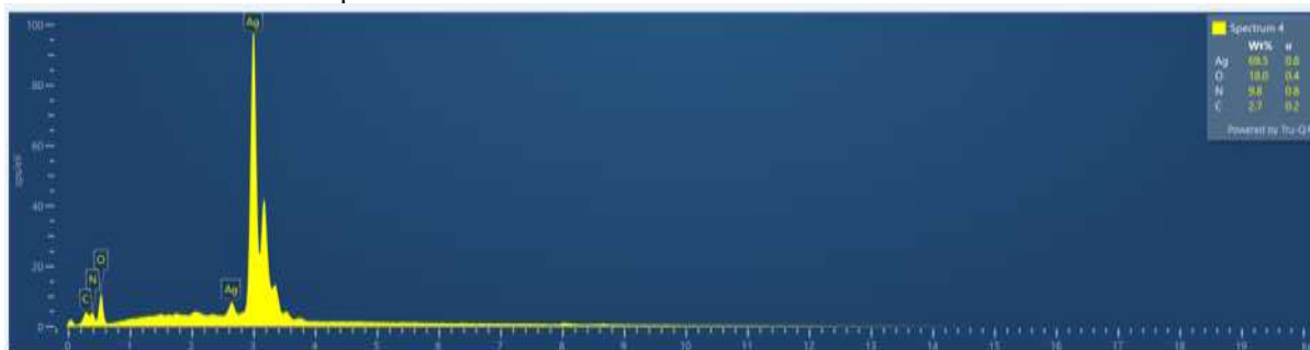
Figure 1: EDX spectrum of the biosynthesized silver nanoparticles (AgNPs). The peak at 3.0 keV confirms a high concentration of elemental silver at 69.5 wt%. Minor peaks for carbon, nitrogen, and oxygen indicate the presence of organic capping biomolecules from the Andrographis paniculata extract
