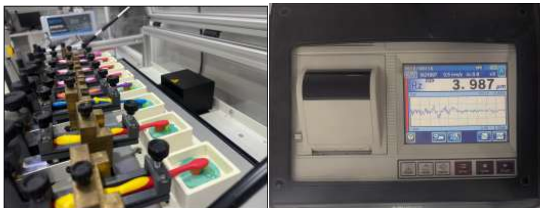
Fig 1a: Brushing simulator (ZM 3.8 SD Mechatronik) used for the toothbrushing abrasion test. Eight extracted primary teeth specimens mounted in acrylic blocks were subjected to 10,000 brushing cycles under standardized load and brushing conditions to simulate approximately one year of toothbrushing. Fig 1.b: Stylus profilometer (Mitutoyo SJ-310) used for surface roughness evaluation. Surface roughness parameters including Ra (average roughness), Rq (root mean square roughness), and Rz (average maximum height) were recorded before and after brushing simulation.
