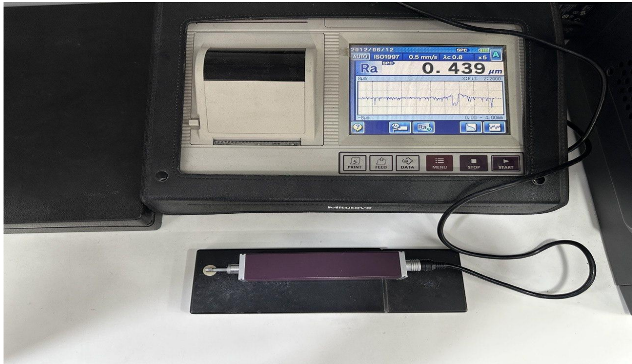
Fig. 2. Stylus profilometer - Mitutoyo SJ 310 used to obtain the values of surface roughness
