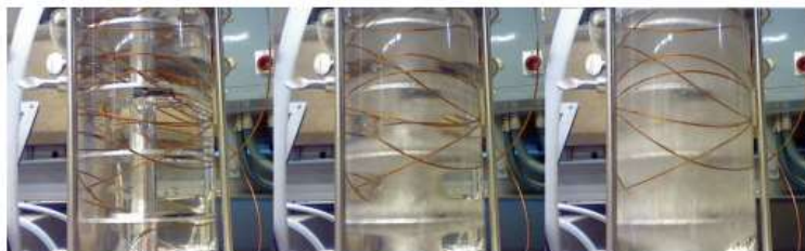
Figure 2: Immobilisation of PCM Throughout Charging
