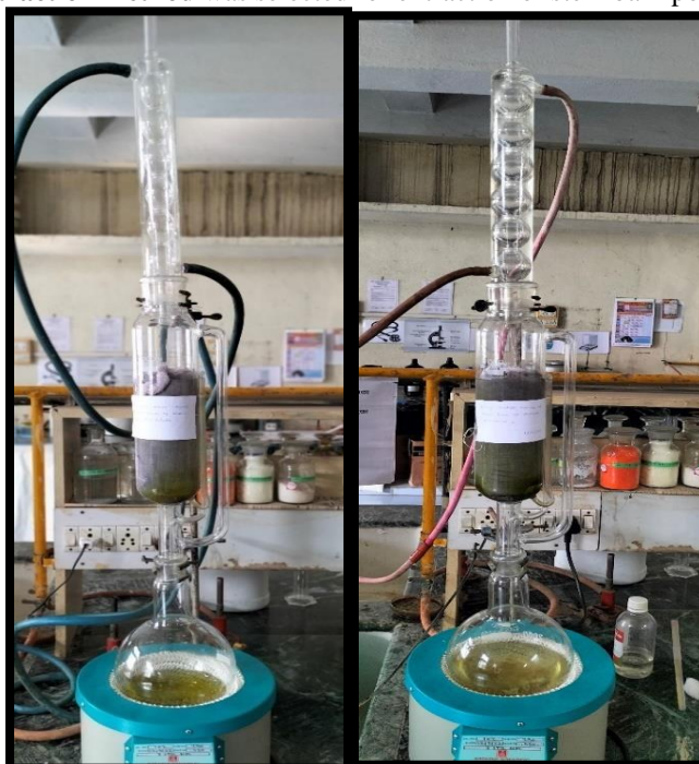
Image No.9: Soxhlet Extraction Ethyl acetate and Methanol Extraction
